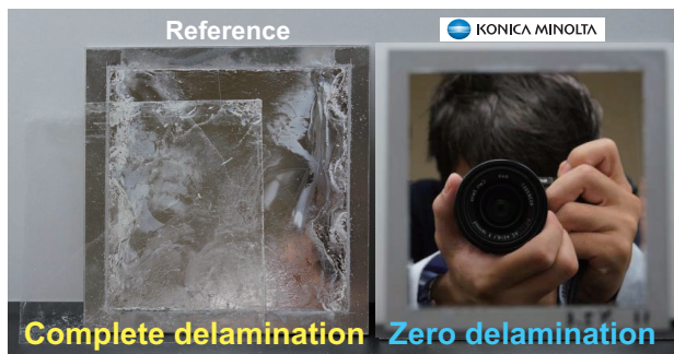
Fig. 8 Salt water immersion test. A mirror using the mirror films of a competitor and one using Konica Minolta's mirror film were soaked in 3.5% salt water. After 21 days, the competitor's mirror had completely delaminated, but after 145 days the Konica Minolta mirror showed no change, thanks to the mirror film's anchor layer.
