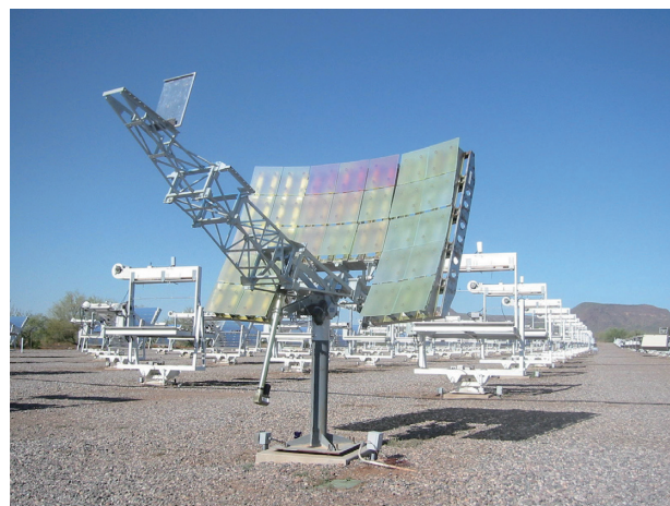
Fig. 3 An ultra-accelerated weathering system (UAWS) was used for testing in the Arizona desert, U.S.A., with the apparatus shown. Our UV energy exposure test, corresponding to 25 years exposure, was achieved in about 6 months 2), 3), 4) .
