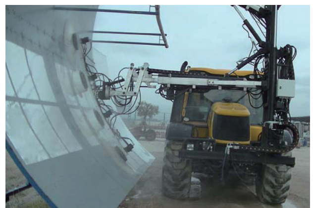
Fig. 10 Konica Minolta's cleaning method on a large scale. Our brushes have been mounted on vehicles and used in actual trough cleaning 9) .
